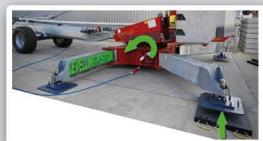
**Simplified levelling:** Thanks to specifically positioned stabilizers, base levelling is completed fast and safely, without needing jacks or any other equipment.
