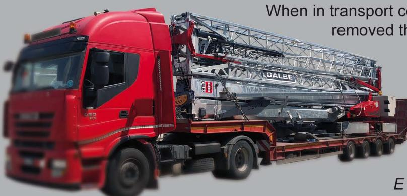
When in transport configuration, **DB 747** weighs 25.9 t: 4 t can be easily removed thanks to two removable 2 t blocks, reducing the total crane weight down to 21.9 t. And its dimensions are suitable for regular transportation.
