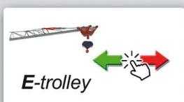
**E-trolley:** Encoder-managed trolley position, a single calibration automatically sets slowing and stopping positions for all jib layouts, with extreme precision.
